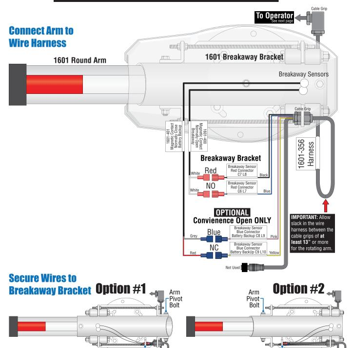
**IMPORTANT:** To secure wires to bracket, allow for some slack in the wires to account for the arm pivoting when arm "Breaks Away" from bracket. Test breakaway feature to **make sure** there is enough slack in the wires when securing wires.
