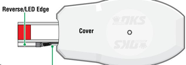
Push stopper against reverse edge and tighten it so edge does **NOT** slide in slot.
