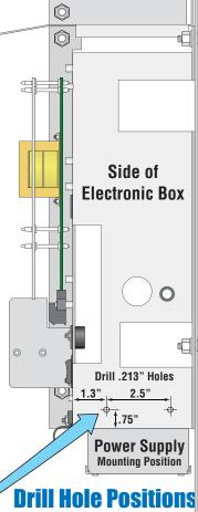
Drill holes in positions shown to mount power supply to side of electronic box.
