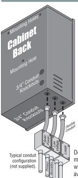
Position the control box on the wall, close enough to the gate operator so the primary operator cable can be easily routed inside the box. Use appropriate hardware (not supplied) in the existing 3 mounting holes to secure the cabinet to a vertical
