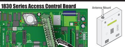
900 MHZ Antenna Options P/N 1514-079 900 MHZ Wireless 900 MHz Antenna Kit P/N 2332-080 P/N 1514-019 Range is Up to 1500 ft Range is Up to direct-line-of-sight Range is Up to 1500 ft **1500 ft** direct-line-of-sight. See instruction sheet for direct-line-of-sight.
