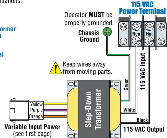
Double check your chosen input voltage plug **BEFORE** applying power to the step-down transformer. Failure to choose the **CORRECT** input voltage plug for your desired input voltage **WILL damage** operator and **VOID** warranty.
