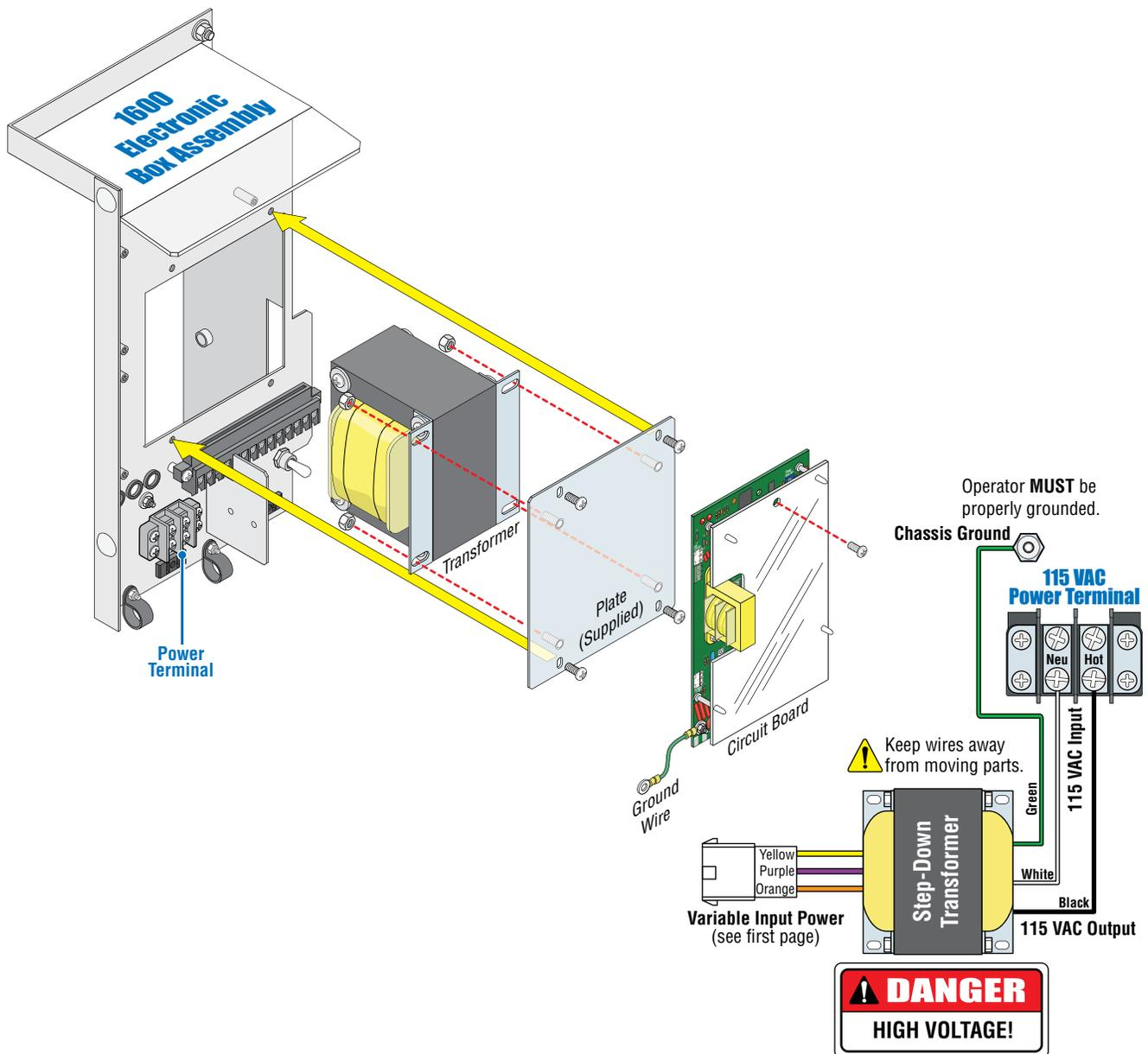
Double check your chosen input voltage plug **BEFORE** applying power to the step-down transformer. Failure to choose the **CORRECT** input voltage plug for your desired input voltage **WILL damage** operator and **VOID** warranty.
