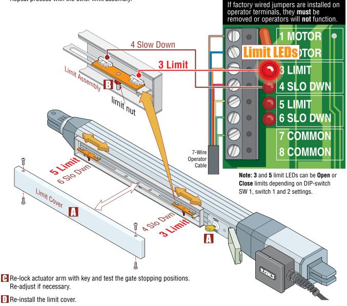
Adjust the secondary actuator limit sensors if dual actuators have been installed. DIP-switch SW 1, switch 2 controls secondary actuator opening direction. DIP-switch SW 1, switch 7 MUST be ON when using dual actuators.
