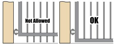
Gates shall have smooth bottom edges, with vertical bottom edged protrusions **NOT** exceeding **0.50 inches**.
