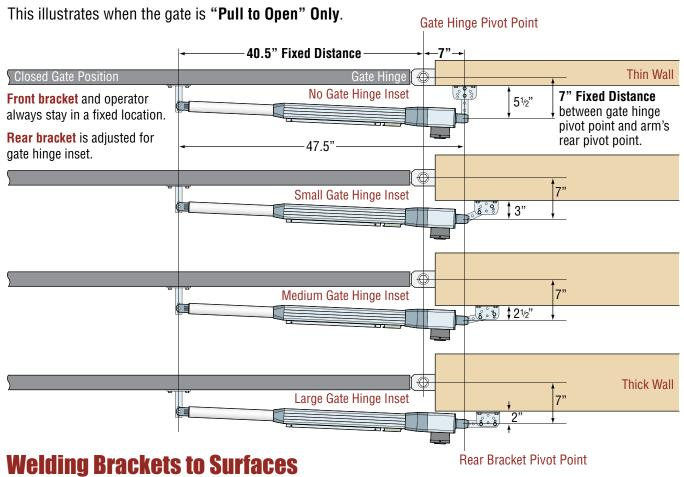
If brackets are going to be welded to the gate and/or wall, only tack weld the brackets with the arm attached. Protect the arm from welding sparks during tack welding. Remove arm before completely welding around the brackets. Make sure the brackets are level when tack welding them! The arm will not operate properly if not level.
