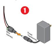
Un-plug power transformer from wire harness.
