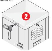
Un-screw wire guard and remove wire harness from operator.
