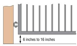
If bottom of gate is 6" to 16"above the ground at any part of the gate's traveling path, entrapment protection for this area is required.
