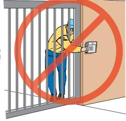
Opening device MUST be mounted a minimum of 6 feet from the gate and NOT accessible through the gate!
