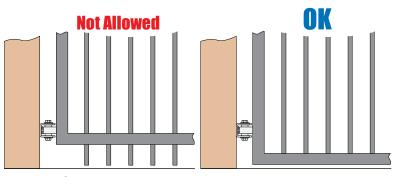
Gates shall have smooth bottom edges, with vertical bottom edged protrusions not exceeding 0.50 inches.
