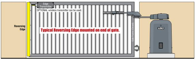
**OPENING Reversing Edge:** Obstructed open-direction reversing edge will **Reverse** the gate **2 inches** and **STOP.** Another input is needed to open the gate.
