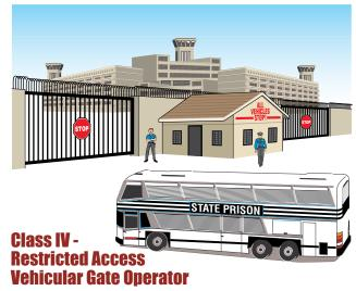
A vehicular gate operator (or system) intended for use in a guarded industrial location or building such as an airport security area or other restricted access locations not servicing the general public, in which unauthorized access is prevented via supervision by security personnel.
