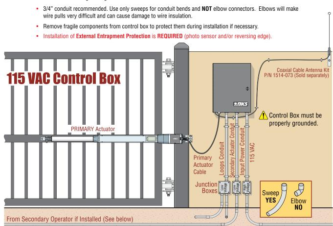
**Dual Actuators Connection (115 VAC or Solar)**
