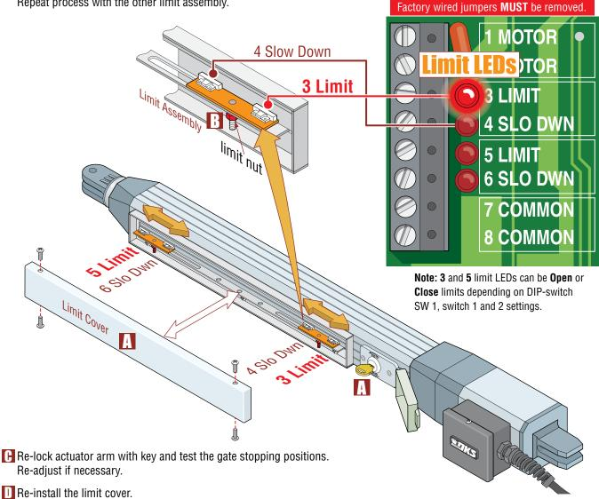
Adjust the secondary actuator limit sensors if dual actuators have been installed. DIP-switch SW 1, switch 2 controls secondary actuator opening direction. DIP-switch SW 1, switch 7 MUST be 0N when using dual actuators.
