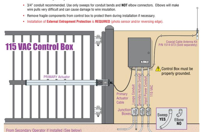
Dual Actuators Connection (115 VAC or Solar)
