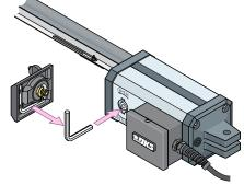
Use key to unlock and remove the cover. Remove allen wrench from inside of cover.
