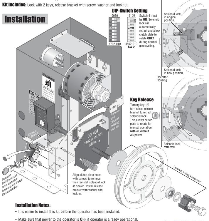
· When reinstalling solenoid lock, existing mounting holes may need to be
