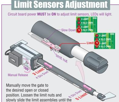
**DO NOT** cycle operator before limit sensors and DIP-switches have been adjusted, damage could occur to gate and operator.
