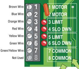
**Operator Terminal Note:** The 8-pin terminals can be unplugged from circuit board for easy wire connections.
