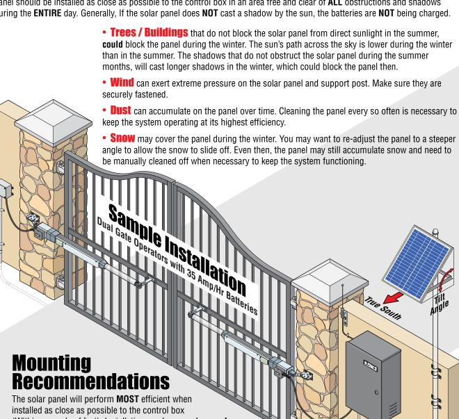
installed as close as possible to the control box
