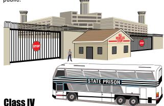
A vehicular gate operator (or system) intended for use in a guarded industrial location or building such as an airport security area or other restricted access locations not servicing the general public, in which unauthorized access is prevented via supervision by security personnel.
