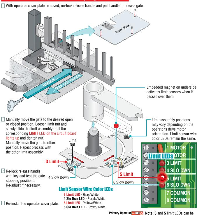
Adjust the Secondary operator limit sensors if dual operators have been installed. SW 1, switch 2 controls secondary operator opening direction. SW 1, switch 7 MUST be ON when using dual operators (See page 19).
