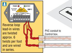
Exit and Reverse Loops Note: Low current draw external exit and reverse loop detectors are used in place of the plug-in exit and reverse loop detectors to maintain power to these loops at all times. Circuit board shuts down power to plug-in loop detectors when not in use (idle time).
