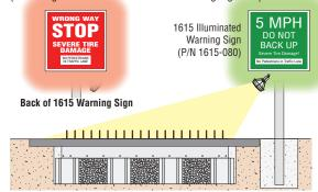
Additional lighting, warning signs and pavement markings can be used to increase awareness for potential danger and to separate pedestrians from vehicular traffic.
