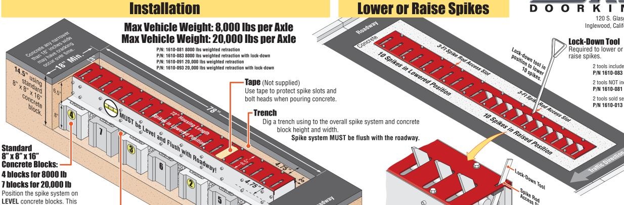
Load gravel inside the trench up to the top and inside the holes in the concrete blocks. This will help the drainage process and avoid soil run-off underneath roadway. **Attaching Lock-Down Tool to Spike Rod**
