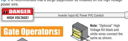
12 AWG copper wire To gate operator (High Voltage) Operator High Voltage PVC Conduit Operator Low Voltage PVC Conduit To gate operator opening device's terminal (N.O.) and (Com).
