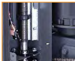
limit switches direct driven and easily adjustable
