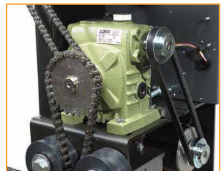
full size gearbox heavy-duty 30:1 ratio gearbox
