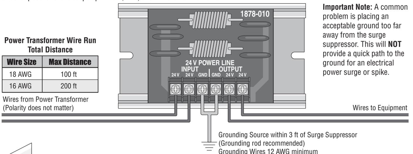
**Important Note:** A common problem is placing an acceptable ground too far away from the surge suppressor. This will **NOT** provide a quick path to the ground for an electrical power surge or spike.
