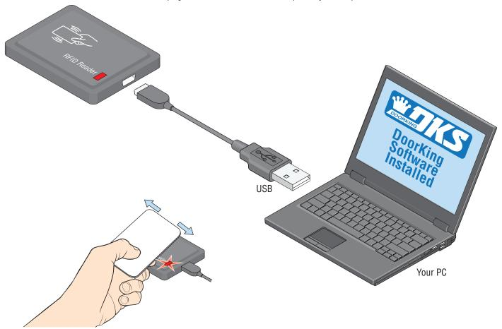
Wave the card above the reader to read card code. LED will flash.
